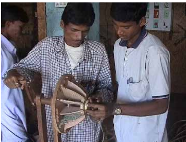
Kailash trying coil technique on spindle machine
