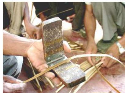
Sandpaper pad used to finish bamboo strips
